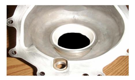
7. **Caution!** Care must be taken to avoid damage to the bearing race while filing. A coffee cup can be used to cover the bearing race.
