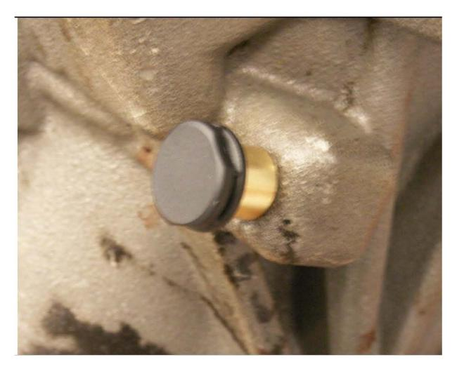
15. If the angle <u>gear</u> does not have the improved vent in place, as shown, install new bleeder pipe and filter.
