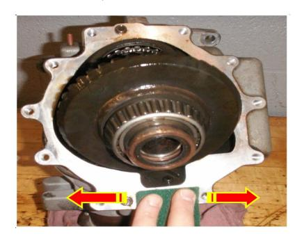
**Note!** Use the abrasive cloth radially, along the flange.
