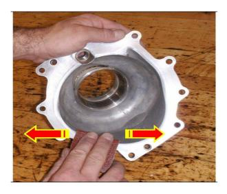
**Note!** Use the emery cloth radially, along the flange just as the arrows indicate. 10. Clean out filing swarf.
