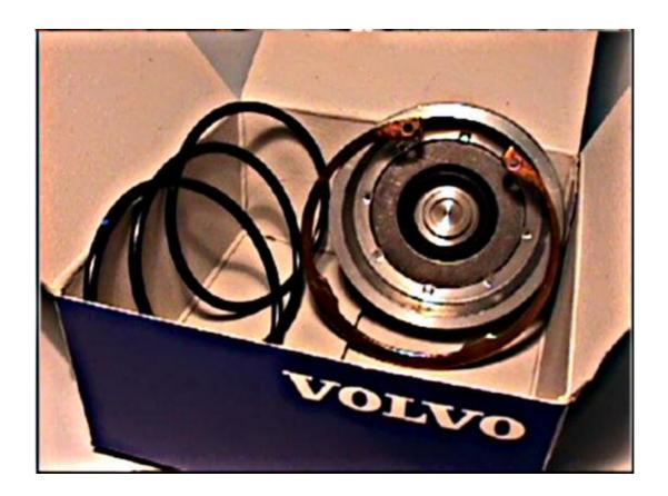
Install two of the O-rings from the kit (PN 30651771) onto the new cover. Lubricate the O-rings with transmission fluid.
