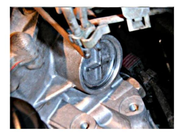
The cover is a tight fit, so it will usually stay in the transmission even after the snap-ring has been removed.
