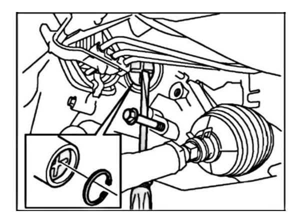
Once the new cover is placed in the bore, push it in using the bolt and screwdriver (this is to compress the spring). Install the new snap-ring and be sure it is properly seated in the groove.
