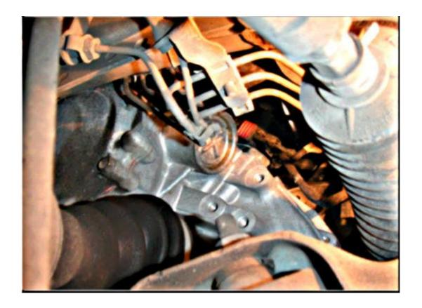
Remove the bolt, clean up any spilled oil, re-install the splash pan and the LF wheel.
