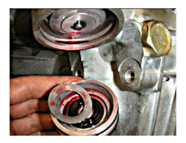
Remove the servo cover from the transmission. If it is faulty, it will look like the one pictured here. The steel washer will have become separated from the aluminum cover. As pictured here, the piston and spring will usually stay inside the transmission. If the piston begins to slide out, push it back in and it will usually stay in place.
