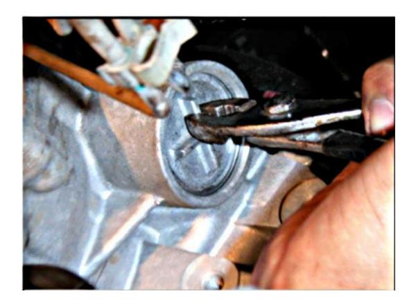
Gently twist the cover so that it rotates a bit in its bore. Once it is free, it will easily come out of the transmission <u>case</u>.
