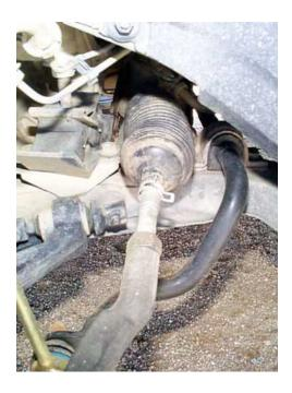
4) Remove the 18 mm bolt that holds the outer tie-rod end to the hub assembly.
