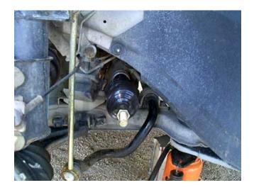
4) Now put the nut onto the inner tie rod end. I used the old tie-rod end to place the nut in approximately the same distance as the old tie-rod stop nut was when I took it out.
