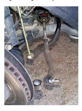
6) Now for the inner tie-rod end. I didn't have a wrench big enough to fit the inner tie-rod end so I used a small pipe wrench. You can see the flats for a wrench just in front of the red plastic bushing.
