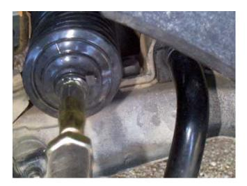
6) Screw the outer tie-rod end (new one I hope) onto the inner tie-rod end up to the nut. When you hit the nut tighten the nut by holding the outer tie rod end (there are flats on it) and the nut together. After tightening it up, turn the outer tie rod end so the stud faces down.
