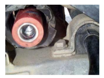
Here is the inner tie-rod out of the car. The ball joint in mine had about a 1/16" of slop (wear) in it.
