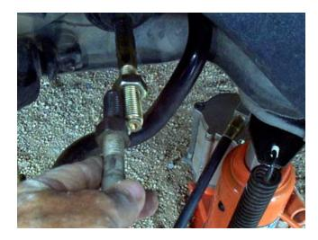
5) Now comes the only real tricky part of this repair. You have to work the boot over the end of the machined surface of the steering rack. It is a real PITA (ask your dad, if you don't know this acronym) but doable. When you get the boot over the end of the steering rack, work the cable tie over it and cinch it up tight. Finally clip the excess cable tie off.
