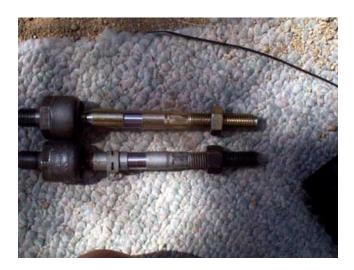
2) Slide the new boot over the tie-rod end with the large end of the boot facing the ball joint of the tie-rod end. After you get the boot on the inner tie-rod end, push it as far forward as you can get it (toward where the nut will be put on ).
