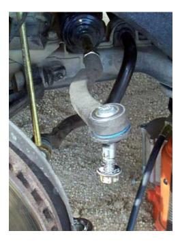
7) Reattach the outer tie-rod end to the wheel assembly and tighten the 18 mm nut to (torque value?).
