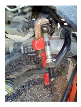
Lay down underneath the car and give it (the wrench or the pipe wrench) a yank in a counter clockwise direction. It will break loose fairly easily. After a turn or two, you'll be able to remove it by hand, simply by unscrewing it. You can see the remains of the bellows in this picture.
