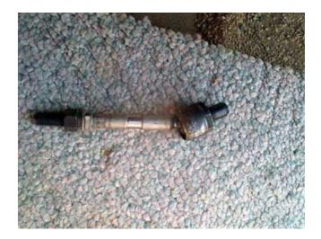
I then knocked the inner bellows clamp off with my 12" punch and a hammer (the replacement kit comes with the clamps). Disassembly is almost complete.
