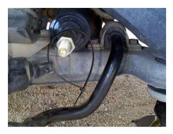
Repeat this with the outer end of the boot...this is an easy one. Just push the boot to the machined surface (see photo in Step #1 of reassembly) on the tie-rod end and cinch up with the smaller cable tie and trim off the excess.
