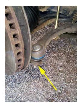
Note: After removing the nut, whack the side of the assembly with the BFH (just about where the arrow points to). Now remove the shaft from the assembly.
